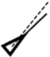
If an AIS target (activated or not) is calculated to pass preset CPA and TCPA limits, it will be classified and displayed as a dangerous target and an alarm will be given.
