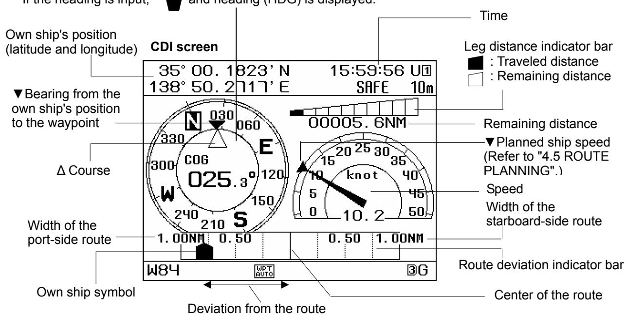
The highway screen displays information in Course Up mode while the own ship's position is fixed, so the route turns when the own ship turns. As a result, the route may not be displayed depending on the course.
