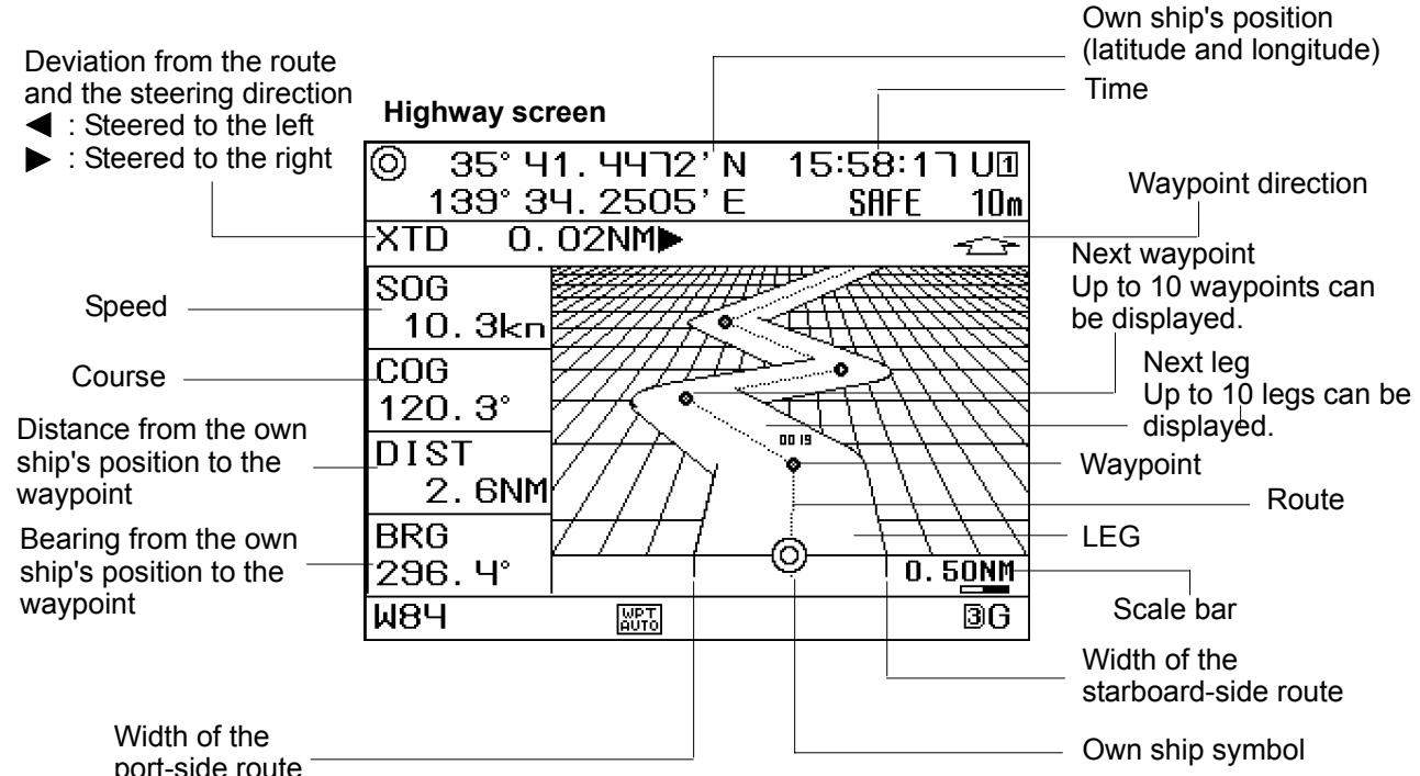
The highway screen's scale can be changed by pressing or . The scale width is the same as the plot screen's. Please refer to "4.3.3 Zooming the Screen In and Out".
