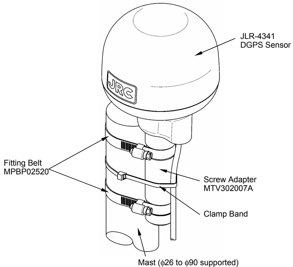
1. Loosen the fitting belt screw with a screwdriver to remove the clamp.
