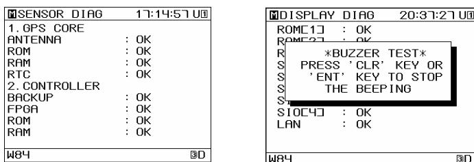
After self-diagnosis has been performed for the screen, the entire screen is highlighted repeatedly such as black to white, white to black. Check if some dots are omitted.
