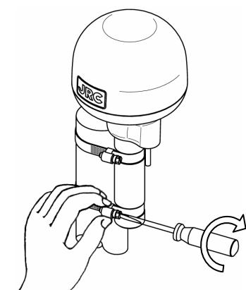
How to Install the Sensor on the Mast
