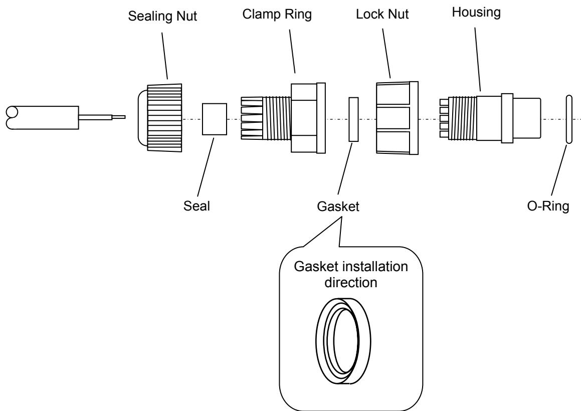
Clamp Ring tightening torque: 1.2 - 1.5 kgf-cm
