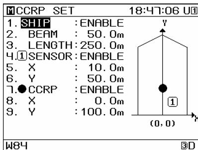
The CCRP position can be received. If the set position and received position differ, the following alert will occur, so please perform the settings again. A "\*" will appear on the status bar until the settings have been redone.
