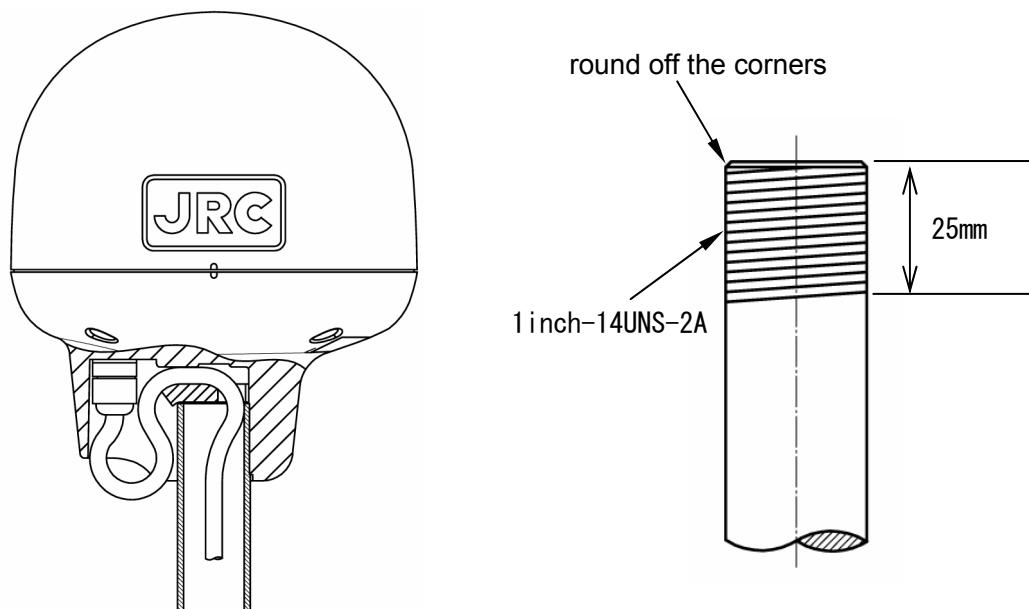
(4) When performing attachment, always hold and turn the sensor base. Holding and turning the radome may result in a large amount of force applied at the junction of the base and the radome, resulting in damage to the sensor.
