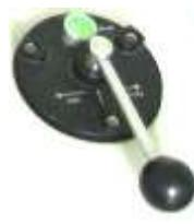
Switching from manual to automatic control push button . The autopilot remembers the course at which automatic control is enabled.
