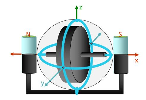
If we imagine that the north axis is turned eastwards when the gyrosope is started, ths axis will be raised when the Earth rotates toward east.
