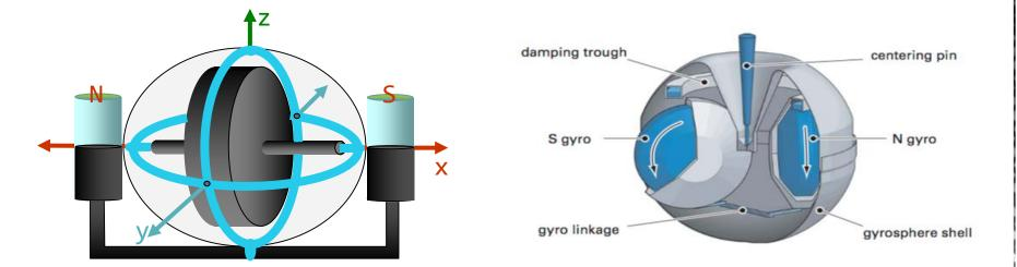
In order to obtain a force that can precess the gyro axis toward north, a container with mercury is mounted on the axes. The system is called mercury or Hg control.
