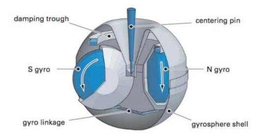
Gyrocompass will have some common elements that can be characterised as:
