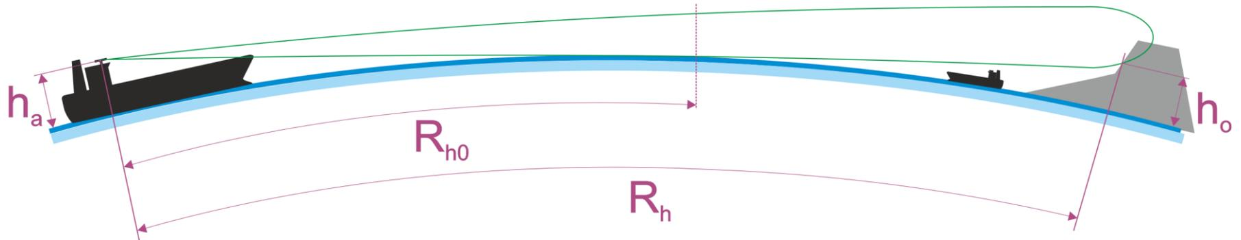
the ability to detect objects, beyond the horizon, depends on the height of the antenna and the height of the detected object. This corresponds to the formula:
