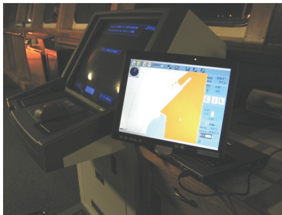
Figure 6. Pilot navigation system (portable version) built at the Maritime University of Szczecin.
