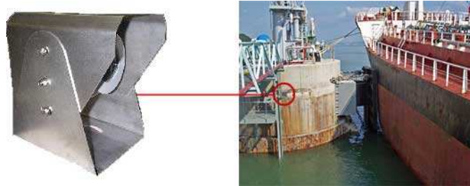
Fig. 1. External sensors of the SmartDock Harbour Marine-made system (Trelleborg www)
