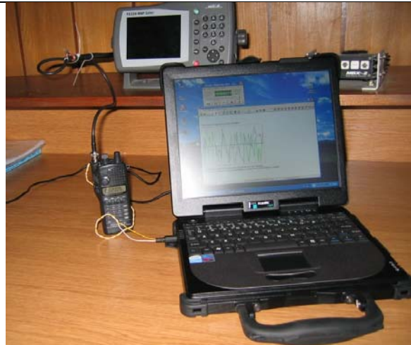
Fig.7 Kenwood TH28 handheld scanner with application for AIS decoding during tests
