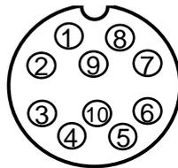
External monitor and alarm output connector pin assignment
