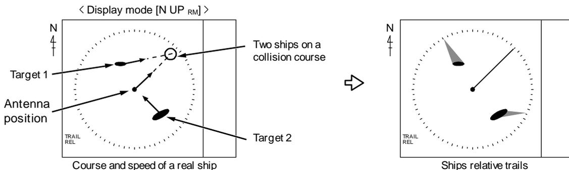
Target 1, whose trail is overlapping the EBL, is a dangerous target while the Target 2 is not. If trail setting is six minutes, and if the trail length is equal to the distance between the antenna position and Target 1, then the collision will occur after six minutes.
