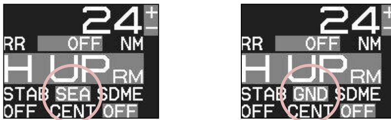
When SDME or EPFS is not available for any reason, it is possible to get the speed over ground by setting reference target.
