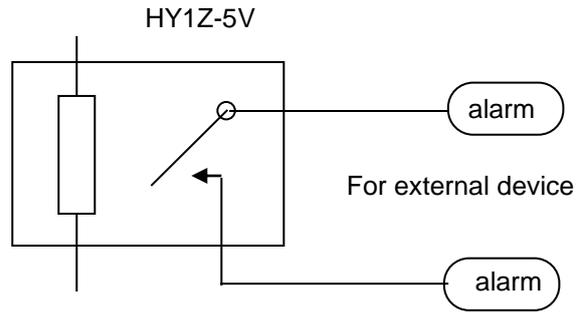
**Note:** Alarm contact will close in case of failure.
