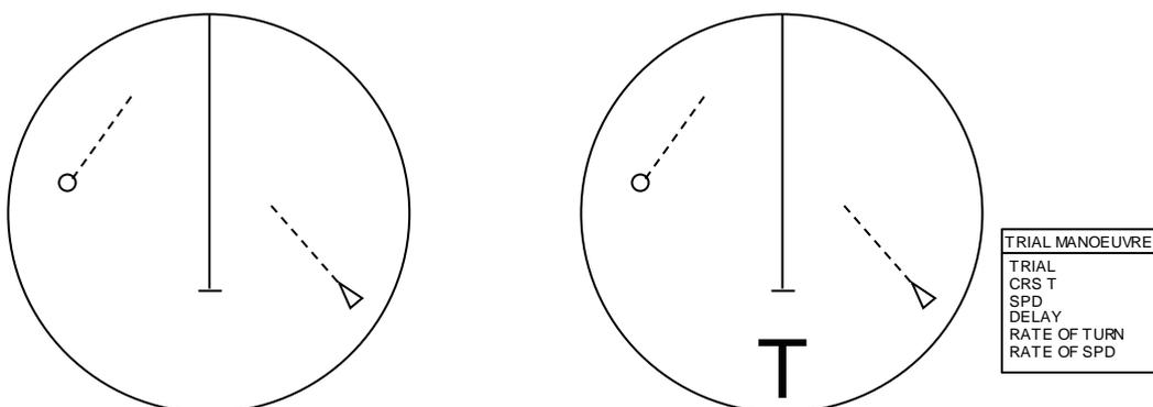
In addition, the movement of the own ship and the other ships is displayed in vector after elapse of the time set at [DELAY] of TRIAL MANOEUVRE setting menu.
