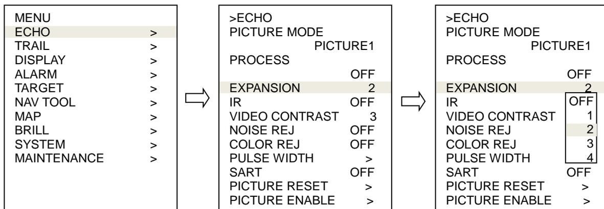
Note: "Menu" setup value is stored in the non-volatile memory inside the radar. Therefore, no setup operation is required after power is turned on.
