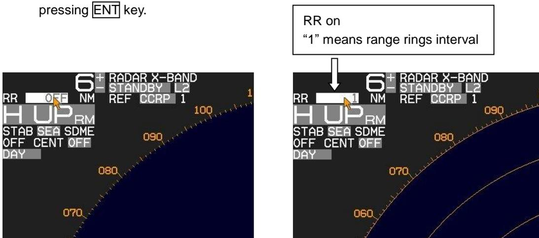
Note: When **[NAV TOOL]** => **[BRG TRUE / REL]** => **[TRUE]** is selected, 0° of the range rings indicates North direction. While, when **[REL]** is selected it indicates heading direction.
