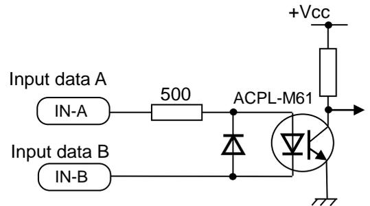
Serial data input circuit
