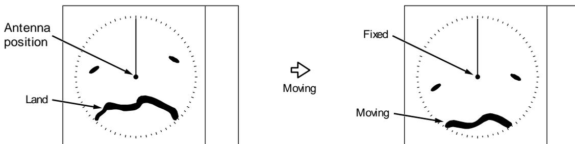
**True motion (TM):** The antenna position on the display moves according to its speed and tidal current. Stationary targets are fixed on the display. This mode is useful to monitor your position with respect to the fixed targets such as land.
