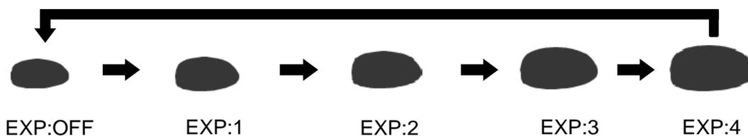
Note: The enlargement of targets has effect on all echoes. So, a large target such as land is also enlarged. Consequently, land and a small target may sometimes be seen as a single target. Pay attention to that.
