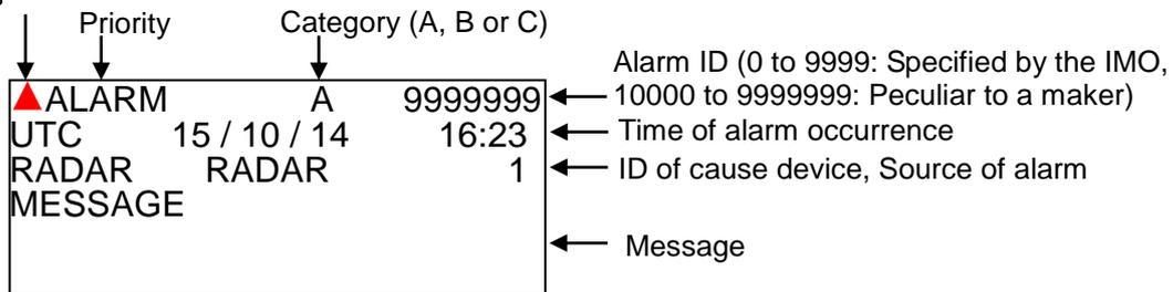
In case of unacknowledged alarm, icon and ALARM of priority will be flashing, and 3 short audible signals will be repeating every 7 sec.
