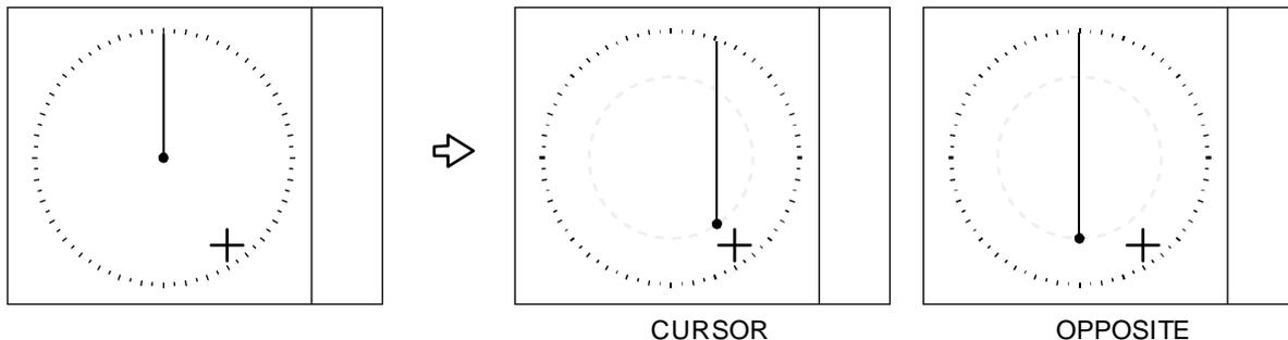
Note: When CCRP is selected for the reference position, there is possibility that CCRP is located outside of 90% echo image area at OFF CENTER function in short range.
