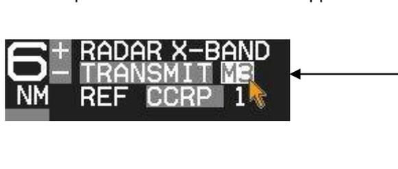
Note: Pulse width can be changed directly at the upper left of the display, with cursor and **[ENT]** key.
