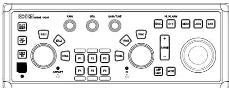
After power on, radar model name and preheating countdown time will appear at the center of the display.
