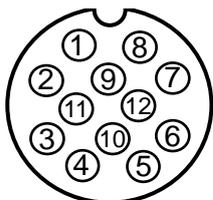
Data connector pin assignment
