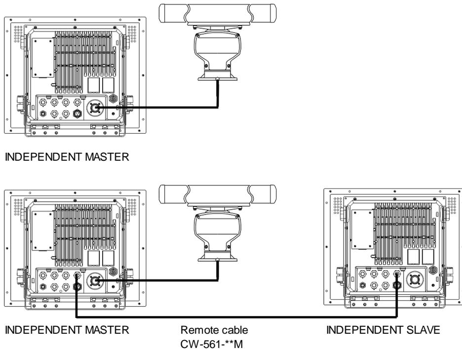
DUAL MASTER: Connection topology is the same as the above-mentioned INDEPENDENT (MASTER) and INDEPENDENT (SLAVE), and the data cable is necessary. By this way, either radar can control the antenna. The radar to which the antenna is connected is DUAL (MASTER).
