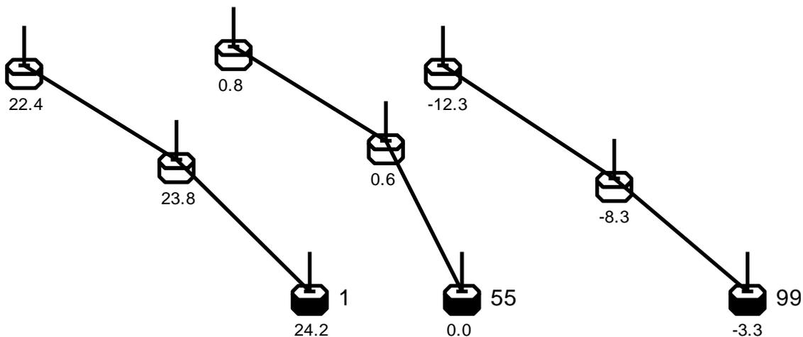
Buoys with same ID will be displayed linked with straight lines. Under each buoy symbol, water temperature can be indicated.
