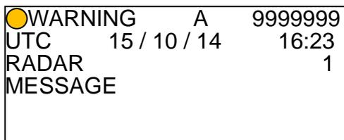
In case of unacknowledged alarm, icon and WARNING of priority will be flashing, and 2 short audible signals will be repeating every 60 sec.
