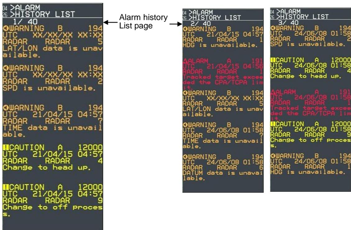
Maximum number of alarms which can be displayed is 200. Alarms in excess of 200 are deleted.
