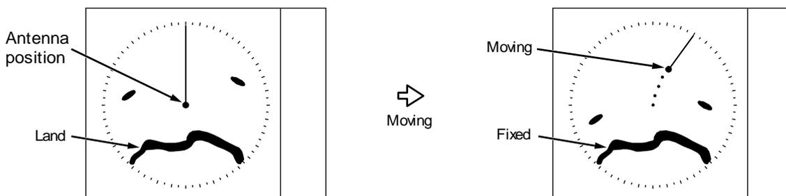
N-UP or C-UP TM mode is selected, own ship position moves to opposite side of heading direction, and begins to show the true motion image. When own ship position reaches center of the range scale, own ship position is to reset to the course over water or to the opposite direction of the course over ground.
