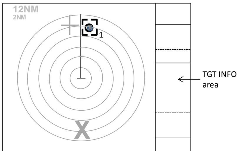
Note: If the parentheses are not displayed, then drag a cursor to the acquisition start symbol and press **ENT** key.
