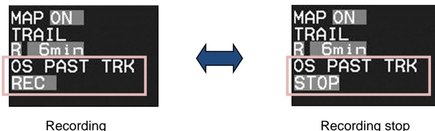
When the recording of the own ship past track is started, move the cursor to the **STOP** of the OS PAST TRK at the lower left of the display, and press the **ENT** key. When the recording of the own ship past track is completed, move the cursor to the **REC** of the OS PAST TRK at the lower left of the display, and press the **ENT** key.
