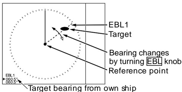
Note: Turning **[EBL]** knob (while pressing it) changes the bearing quickly.
