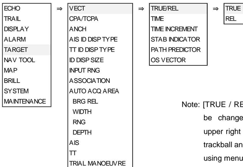
Note: **[TRUE / REL]** and **[TIME]** can be changed directly at the upper right of the display, with trackball and **[ENT]** key, without using menu.
