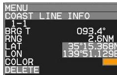
← Edit of LAT/LON data, color setting and delete function can be operated directly using cursor with trackball in this info area.
